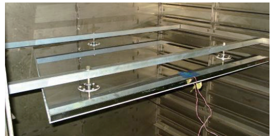
Photo 3 Heat/humidity and thermal shock tests were conducted in a large thermostatic chamber.
